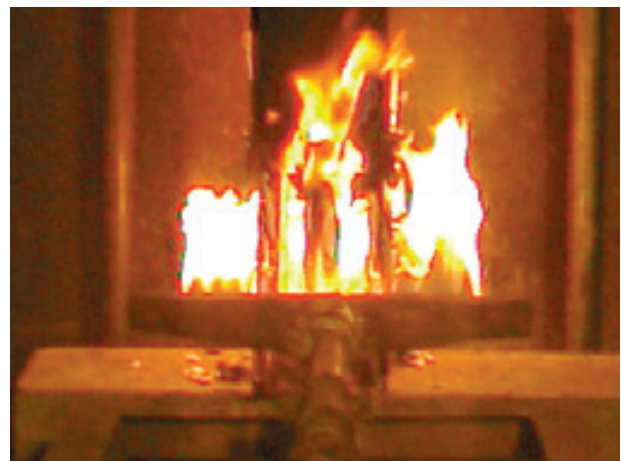
Henikwon Busduct System under ASTA Type Test
