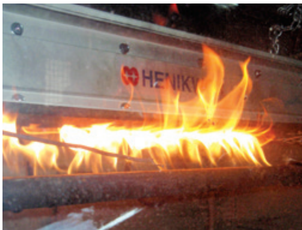
Henikwon Fire-Resistant Busduct System in test chamber burner
